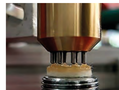
Oiling with a needle metering valve and a special adapter
