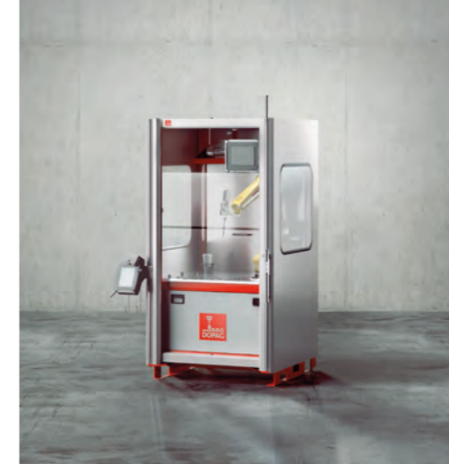
A production cell for potting, bonding and gasketing
