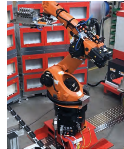
A custom-built metering system for potting: a robot takes over the entire component handling process
